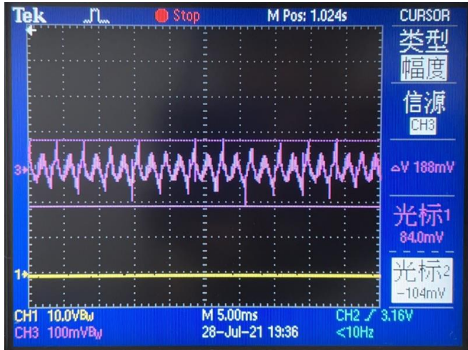
Noise (VIN = 42V, IO = 2.5A, 5 ~ 20MHz bandwidth)
